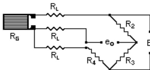
*Fig. 516.3 - Three-wire quarter-bridge circuit.*
