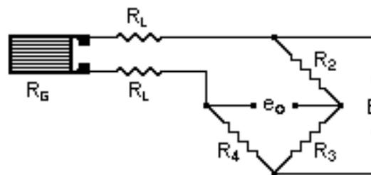
Fig. 516.2 - Two-wire quarter-bridge circuit.
