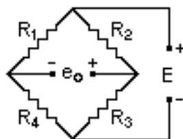
*Fig. 516.1 - Basic Wheatstone Bridge Circuit.*
