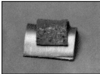
*Water should NEVER be added to RTV silicone rubbers used as protective coatings! In addition to the creation of an excess number of voids during mixing, the quality of the bond between substrate and coating is substantially reduced when water is added. While that effect is desirable when fabricating a conformal pressure pad, just the opposite is needed in a protective coating.*
